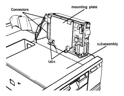
Notice that there are two tabs facing downward on the bottom of the mounting plate. These tabs will fit into two slots in the right side of the subassembly.
